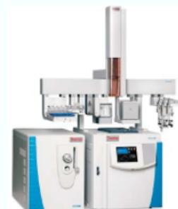
Gas Chhromatograph with mass-spectrometer
