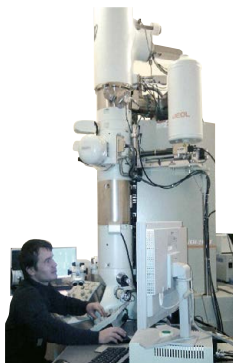
High-Resolution Transmission Electron Microscope JEOL JEM-2100F/Cs/GIF
