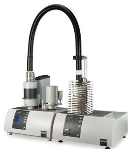
Simultaneous thermal analysis (TG+DSC) system with quadruple mass and IR spectrometers for gases detection
