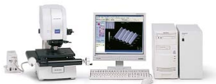
Confocal microscope with implemented video-capture system
