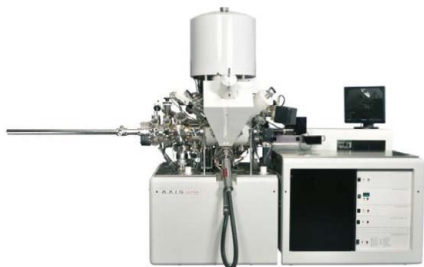
Kratos AXIS Ultra DLD X-ray photoelectron spectrometer
