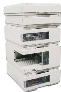
High Performance Liquid Chromatograph Agilent 1100
